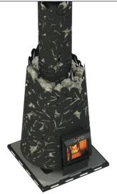
The floor pad protects flooring from hot embers that might fall from the appliance during fuel loading or servicing. The pad must extend at least 200 mm (8 in.) beyond the sides and rear and 450 mm (18 in.) in front of the loading door(s). The floor pad must be a continuous, non-combustible surface.
