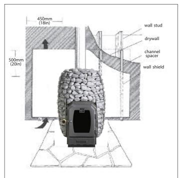
By allowing air to flow between the shield and the combustible surface, a wall shielding assembly can be used to safely reduce minimum clearances. Note that the bottom of the channel spacer is notched to allow cool air to enter.
