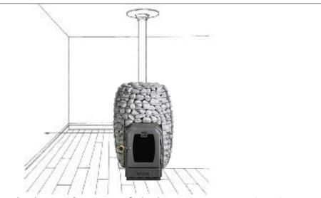
The clearance for an uncertified radiant stove is 1200 mm (48 in.) and for a stove with a sheet metal jacket or casing the clearance is 900 mm (36 in.). The clearances are large because they apply to all shapes, sizes and designs of stoves that have not been tested to determine the actual clearances.
