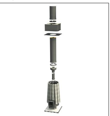
The ideal single-wall flue pipe assembly runs straight up from the stove. Straight venting systems produce stronger draft and will need less maintenance than if the assembly has elbows. A straight single-wall flue pipe assembly needs an inspection sleeve or telescopic section so it can be installed and removed without having to move the appliance. The sleeve also allows some movement for expansion when the flue pipe gets hot.
