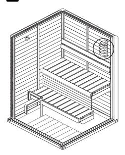
The wall has a pre-drilled hole(s) for the lights. Insert wire(s) to the conduit(s) provided for the lights.
