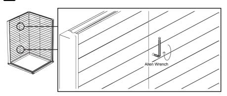
Before moving on to securing the next wall element, make sure that both cam locks are properly secured.
