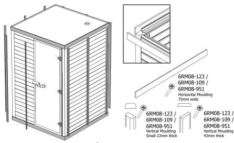
At this stage make sure all internal mouldings are attached as it will be hard to do once the benches are installed.
