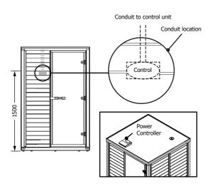
A conduit pipe is provided for the control unit.
