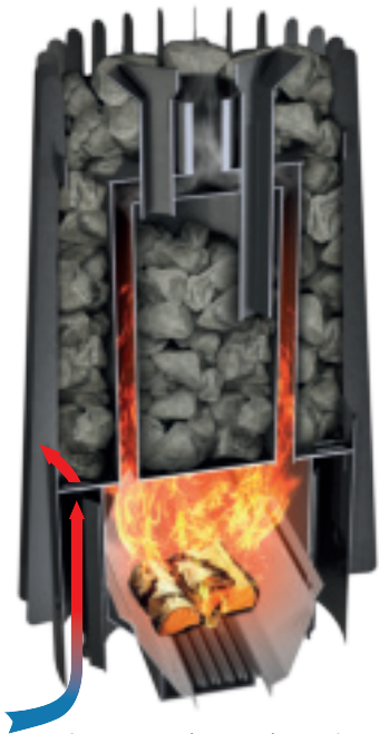
Fig. 3 Heater design and operation
