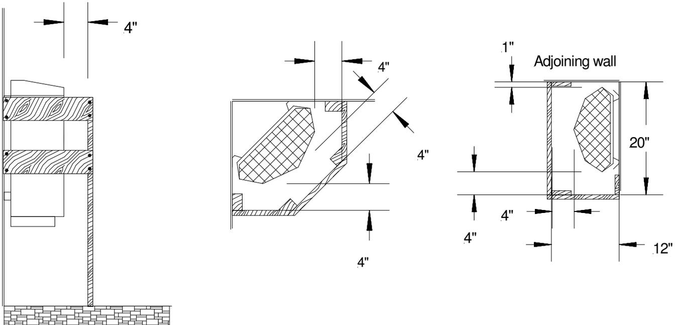
Figure 6. HSH heater guard clearances
